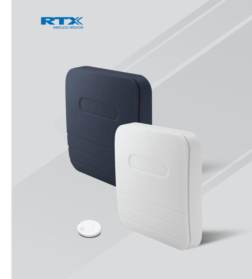
RTX8200 BLUETOOTH BEACON The Bluetooth beacon is used for indoor localization in large building like hospitals, malls, offices or airport terminals. The beacon is placed in the different rooms, or doorways and when a terminal, with BTLE support, detects the beacon it will report the id information to a central sever via the terminals DECT connection. The central server will use this information, based on a deployment plan of the beacons, to detect the terminal location.
